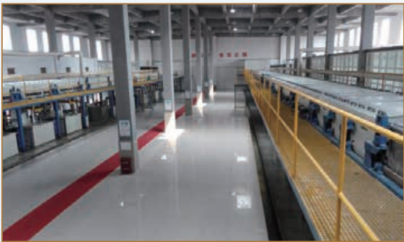
▲ Quality Control A new automatic Digital-control High-speed production line was commissioned in 2015.Data collection and management system at the control room monitors temperature & coating processes,and cutting.
